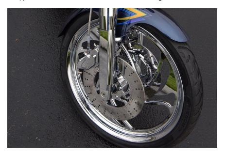
Since the front braking system is the primary brake and supplies as much as 70% or more of the braking power, a dual four-piston caliper, front braking system has been engineered for maximum power. The rear brake system is a single, four-piston caliper design.
