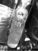
To reach the "ON" position, rotate the ignition switch to approximately the 10 o'clock position. The headlight will come on when the switch has been positioned in the "ON" position.
