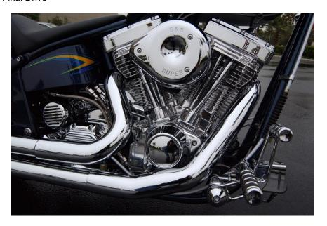
The engine is powered by two large cylinders and combustion chambers that are capable of developing incredible power for a V-Twin four-stroke engine. "Four-stroke" means that each piston moves four times (strokes) for the engine to complete one full cycle.
