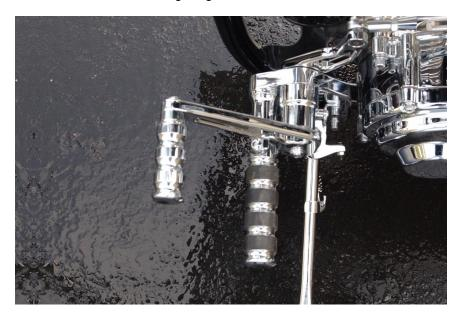
The gear pattern is 1 down, 4 up for the 5-speed and 1 down, 5 up for the 6-speed. The operator must release the foot lever after each gear change to allow it to return to its central position before another gear change can be made.
