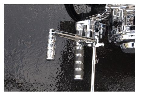
The gear pattern is 1 down, 4 up for the 5-speed and 1 down, 5 up for the 6-speed. The operator must release the foot lever after each gear change to allow it to return to its central position before another gear change can be made.
