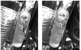
To reach the "ON" position, rotate the ignition switch to approximately the 10 o'clock position. The headlight will come on when the switch has been positioned in the "ON" position.
