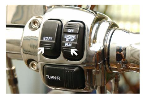
CAUTION: HOLDING THE SWITCH IN THE DEPRESSED POSITION FOR LONGER THAN 5 SECONDS CAN CAUSE DAMAGE TO THE ELECTRICAL AND STARTER SYSTEMS.
