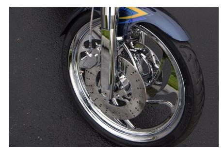
Since the front braking system is the primary brake and supplies as much as 70% or more of the braking power, a dual four-piston caliper, front braking system has been engineered for maximum power. The rear brake system is a single, four-piston caliper design.
