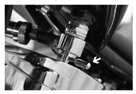
NOTE: IN THE "FUEL ON" POSITION, FUEL ENTERS THE VALVE FROM APPROXIMATELY ONE INCH ABOVE THE BOTTOM OF THE TANK. THE RESERVE POSITION ALLOWS THE FUEL REMAINS IN THE BOTTOM OF THE TANK TO ENTER THE FUEL VALVE.
