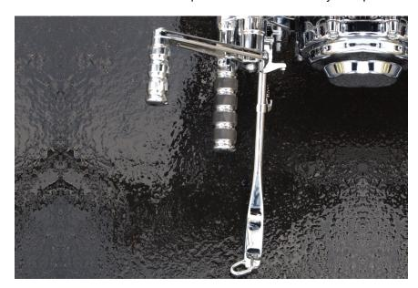
CAUTION: ALWAYS PARK THE MOTORCYCLE ON A LEVEL, FIRM SURFACE; OTHERWISE, THE MOTORCYCLE'S WEIGHT COULD CAUSE THE MOTORCYCLE TO FALL OVER, DAMAGING BOTH THE TANKS AND THE FINISH. A KICKSTAND CAN "SINK" INTO SOFT GROUND, MUD OR HOT ASPHALT.
