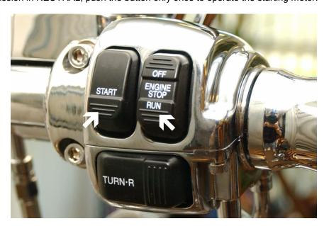
CAUTION: HOLDING THE SWITCH IN THE DEPRESSED POSITION FOR LONGER THAN 5 SECONDS CAN CAUSE DAMAGE TO THE ELECTRICAL AND STARTER SYSTEMS.
