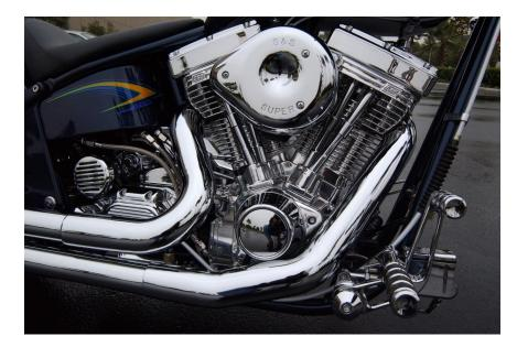
The engine is powered by two large cylinders and combustion chambers that are capable of developing incredible power for a V-Twin four-stroke engine. "Four-stroke" means that each piston moves four times (strokes) for the engine to complete one full cycle.
