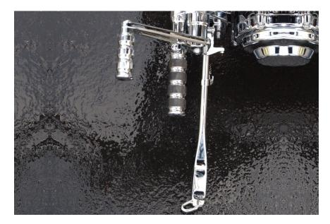
CAUTION: ALWAYS PARK THE MOTORCYCLE ON A LEVEL, FIRM SURFACE; OTHERWISE, THE MOTORCYCLE'S WEIGHT COULD CAUSE THE MOTORCYCLE TO FALL OVER, DAMAGING BOTH THE TANKS AND THE FINISH. A KICKSTAND CAN "SINK" INTO SOFT GROUND, MUD OR HOT ASPHALT.
