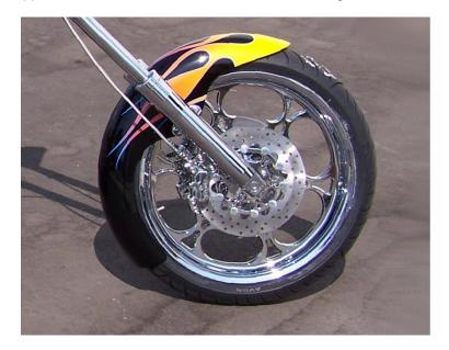
Since the front braking system is the primary brake and supplies as much as 70% or more of the braking power, a dual four-piston caliper, front braking system has been engineered for maximum power. The rear brake system is a single, four-piston caliper design.
