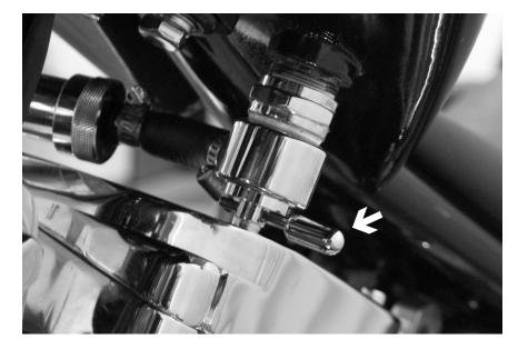
NOTE: IN THE "FUEL ON" POSITION, FUEL ENTERS THE VALVE FROM APPROXIMATELY ONE INCH ABOVE THE BOTTOM OF THE TANK. THE RESERVE POSITION ALLOWS THE FUEL REMAINS IN THE BOTTOM OF THE TANK TO ENTER THE FUEL VALVE.
