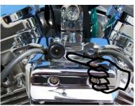
Do not leave the fuel enrichener lever in the ON position after the engine has warmed up or when starting a warm engine. Please refer to the section on hot and cold starting your motorcycle.
