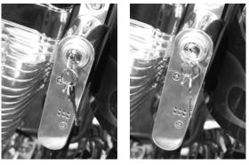
With the key in the center position the electrical system is off but the key cannot be removed.
