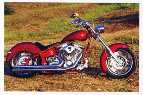
triple-trees. Out back, a Daytec swingarm is cushioned by oil-dampened shocks. Rolling stock is handled with a pair of 18-inch billet wheels with matching rotors and pulley. The rear wheel carries a 250 Avon, while the front runs a 120. Dual four-piston calipers ride up front with a matching rear.
